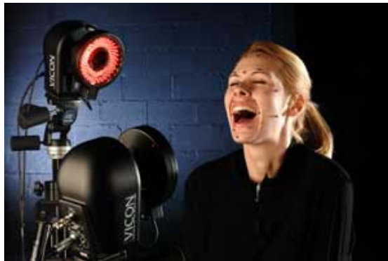
Figure 3: Optical facial tracking (2 cameras)
