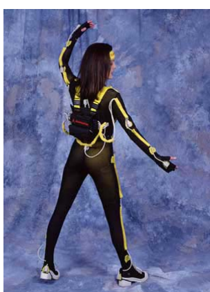
Figure 2: a suit with magnetic sensors in a closed environment
